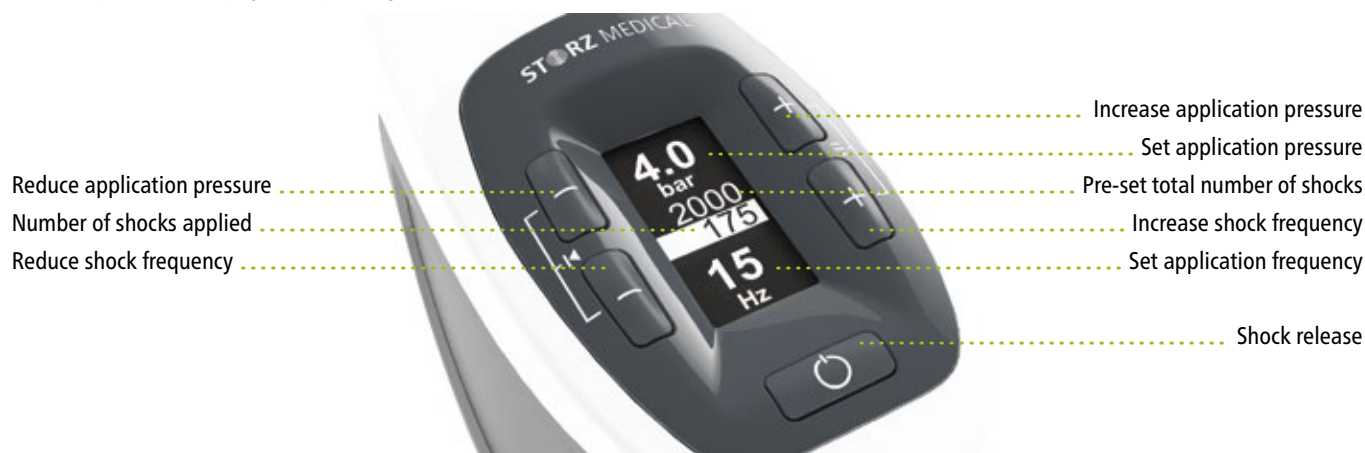
»Active-tip-control« display and operating elements
